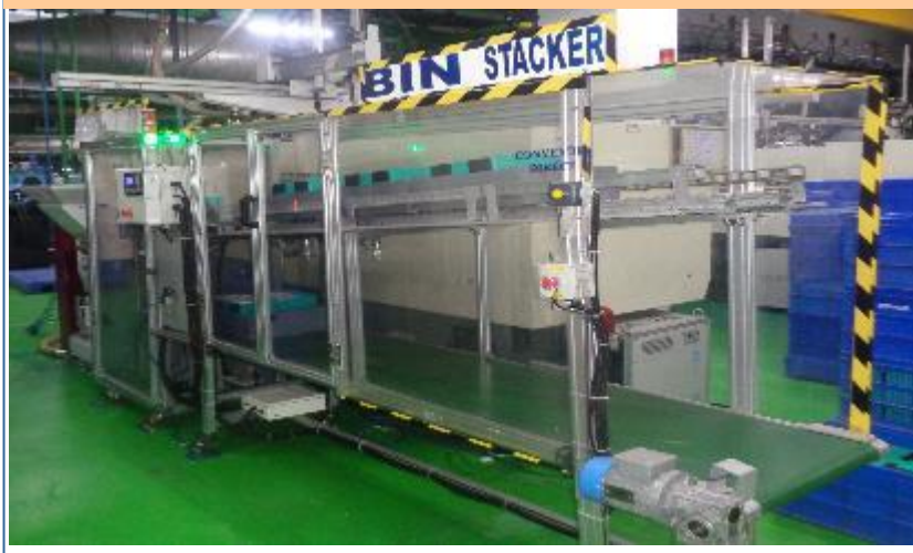
Machine running with Bin stacker conveyor
