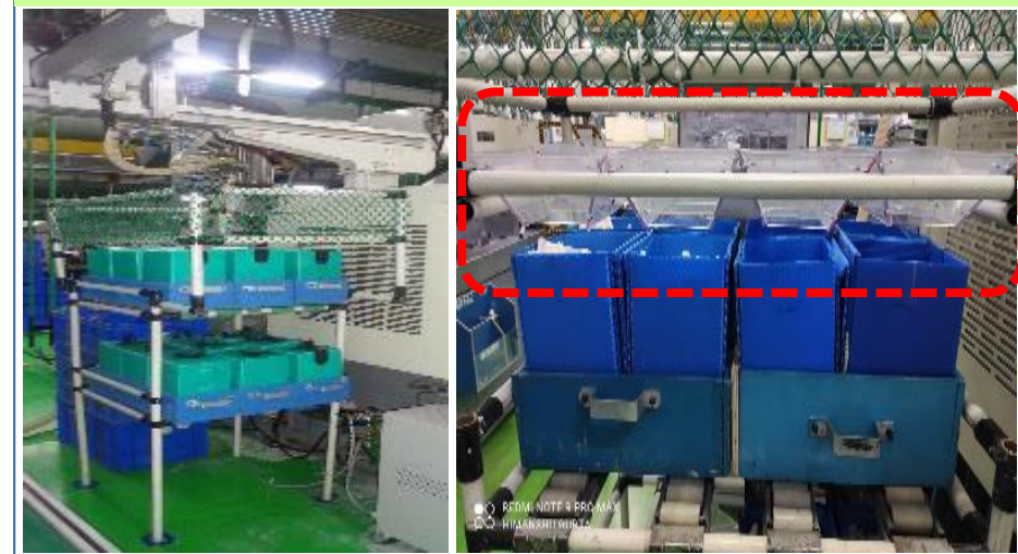
Machine running without bin stacker conveyor with the help of PP box stand
